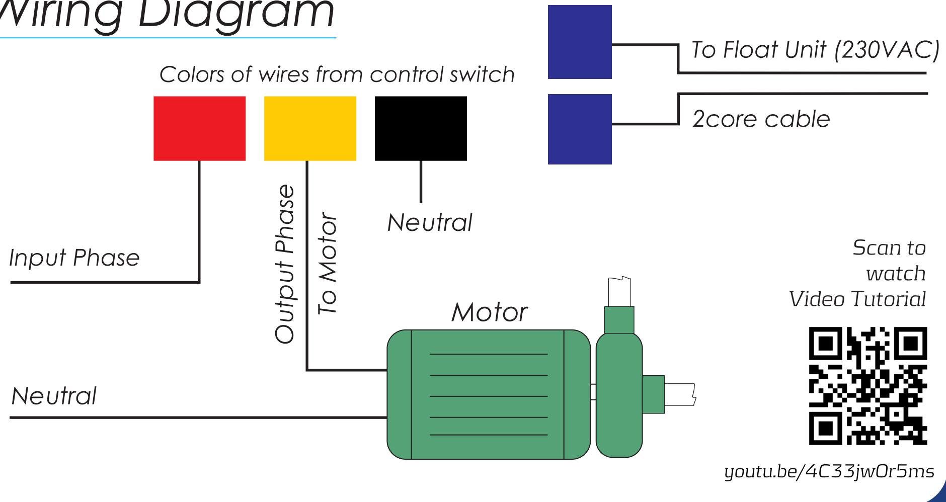
Make the connections as per the above wiring diagram in accordance to the colours of wires from the control unit.
